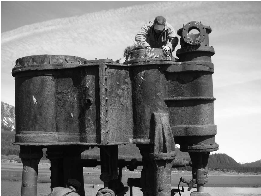
Figure 6. Nautical archaeologist John Jensen confirmed the identity of the SS Portland by measuring the diameters of the engine cylinders. Photo by Dave McMahan.
